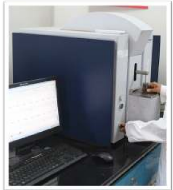
Chemical Analysis by Optical Emission Spectrometer
