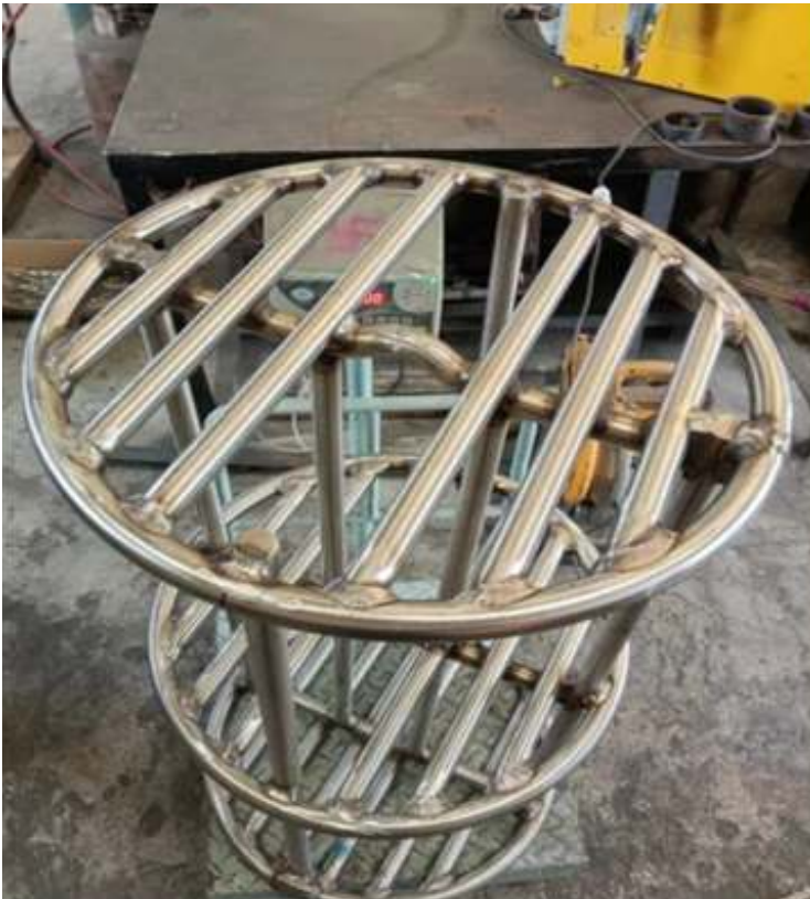
Stainless Steel Charging Tray for Pit Type Heat
